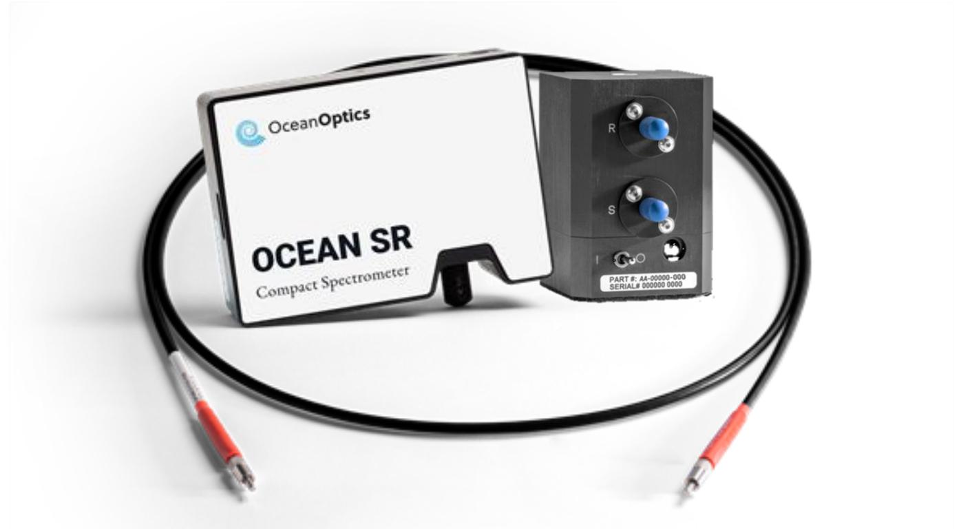
Use the patch fiber to connect the spectrometer SMA port to the lower 'S' port on the integrating sphere.
